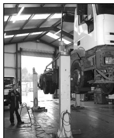
• Truck being lifted using 32 tonne portable hoist
