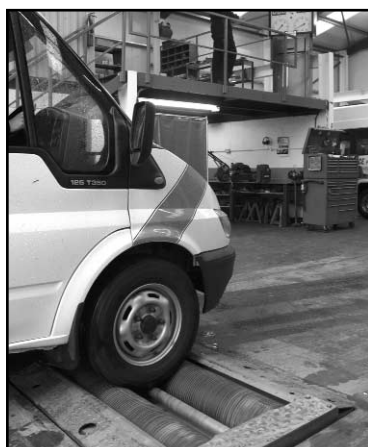
• Technician Oliver Lavery performing break rolling road test
