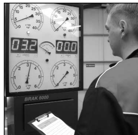
• Technician Oliver Lavery performing break rolling road test
